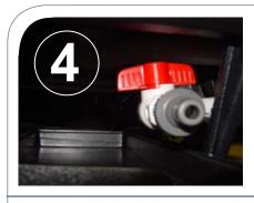
The discharge valve is closed when the valve handle is horizontal.
